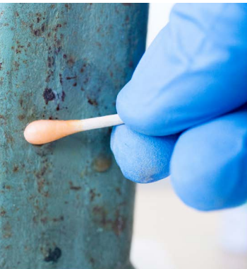
Orange = no chromium-6 Examples of tests on paint layers
